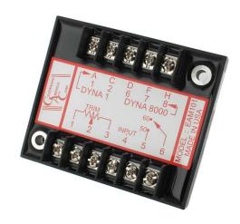
The second terminal block on the EAM101 offers 6 terminals and accepts connections from an external speed trim pot, GAC PIN TP501 or TP503, and signals from the GAC Load Sharing Module, Auto Synchronizer and 50/60 Hz switch.
