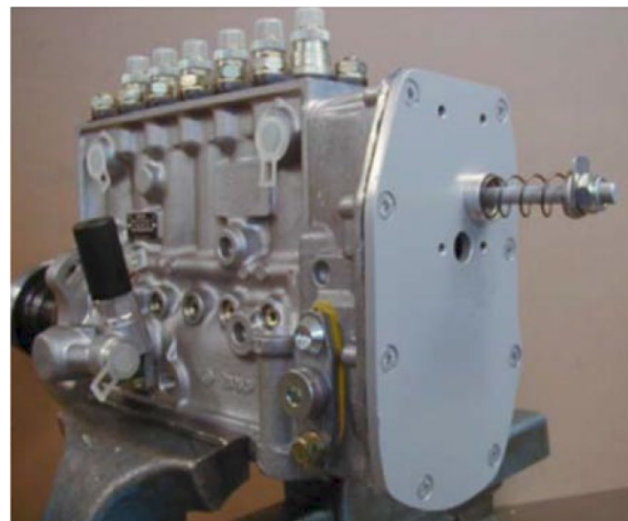
FIGURE 6 ADAPTER PLATE and RACK EXTENSION INSTALLED
