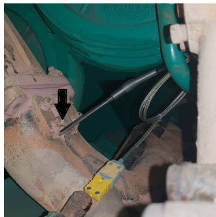
FIGURE 17 INSERT COMPRESSION FITTING WITH SENSOR INTO BUNG
