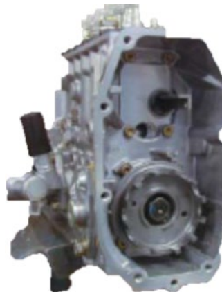
FIGURE 2 REAR GOVERNOR HOUSING REMOVED
