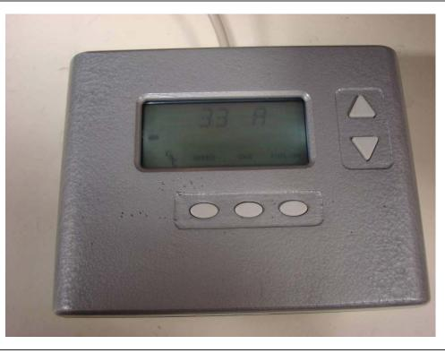
The final real time display is the actuator current on the main display and difference in RPM on the bar graph.
