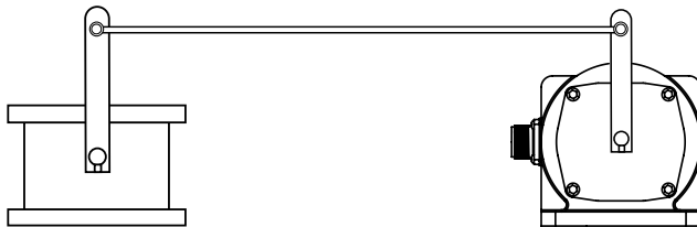
FIGURE 1 FUEL LEVER AT MID FUEL/AIR POSITION
