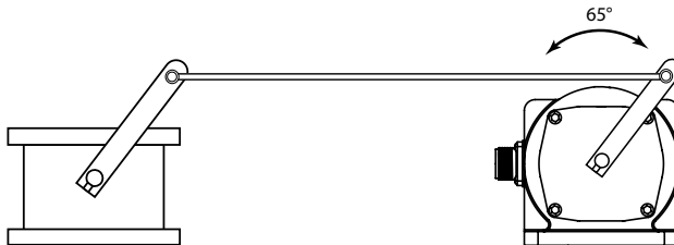
FIGURE 2 FUEL LEVER AT FULL FUEL/AIR POSITION
